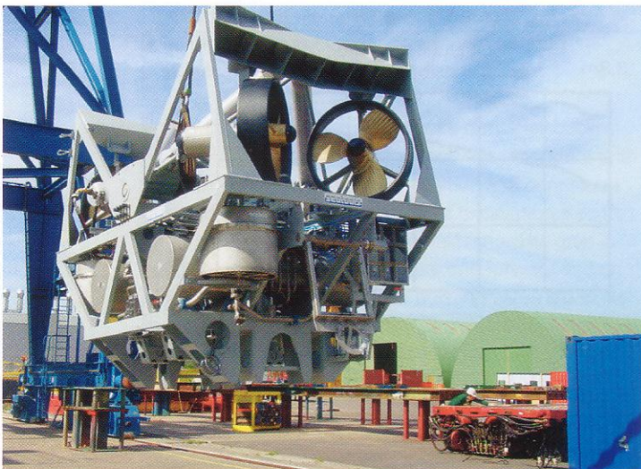
Figure 6. ROV with protective frame before assembly with clamshell.
