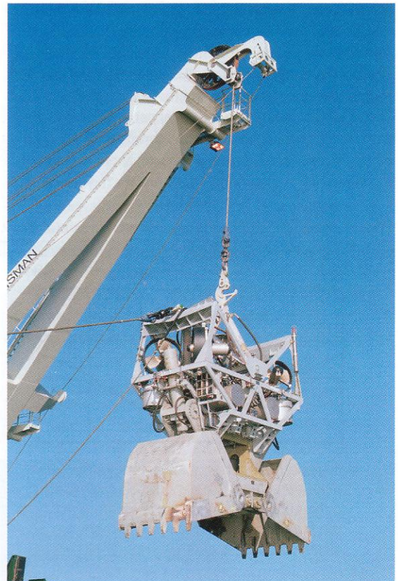
Figure 7. Assembly of clamshell and ROV suspended from A-frame.
